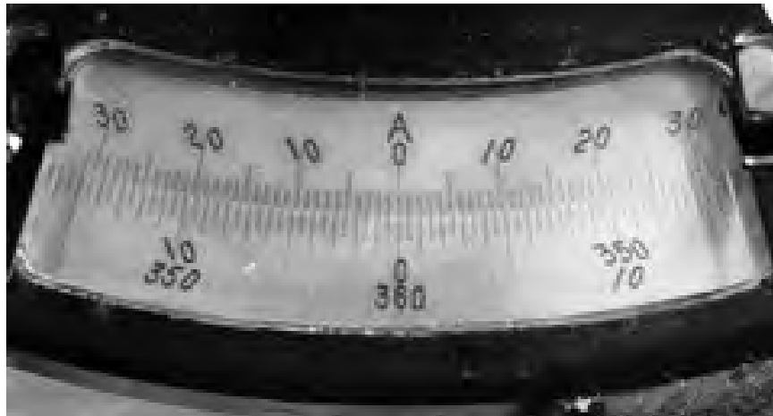
Figure 1-56: One-minute Vernier Set at 0 Degrees
