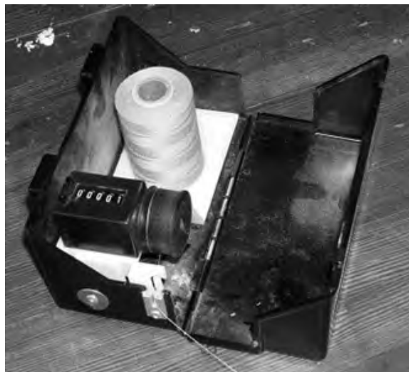
Figure 1-33: String Box or Hip Chain
